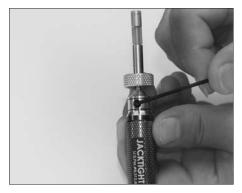
**STEP 1:** Loosen set screw by turning counterclockwise, using the allan wrench located inside the handle.
